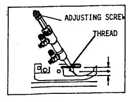
WHEN RE-SHARPENING THE KNIVES, OR CHANGING THE KNIVES OR TAKING OFF THE SPREADER TRIMMER SET IF NECESSARY, PLEASE ASSEMBLE BACK THE SPREADER TRIMMER ACCORDING TO FOLLOWING ITEMS.
